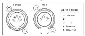
Connect the Console's DMX OUTPUT to the first fixture's DMX INPUT, then the first fixture's DMX OUTPUT to the second fixture's DMX INPUT and so on. It is recommended not to connect more than 32 units on a single DMX universe. On the last fixture's output connect a DMX terminator. (The terminator is a XLR connector with a  $\frac{1}{4}$  W and  $\frac{120\Omega}{120}$  resistor between the pin 2 and pin 3) as shown below:
