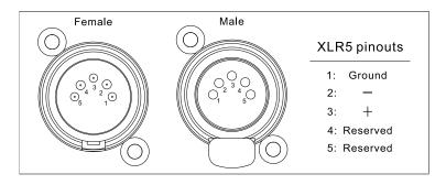
Connect the Console's DMX OUTPUT to the first fixture's DMX INPUT, then the first fixture's DMX OUTPUT to the second fixture's DMX INPUT and so on. It is recommended not to connect more than 32 units on a single DMX universe. On the last fixture's output connect a DMX terminator. (The terminator is a XLR connector with a  $\frac{1}{4}$  W and  $120\Omega$  resistor between the pin 2 and pin 3) as shown below:
