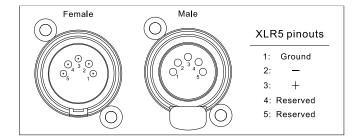
Connect the Console's DMX OUTPUT to the first fixture's DMX INPUT, then the first fixture's DMX OUTPUT to the second fixture's DMX INPUT and so on. It is recommended not to connect more than 32 units on a single DMX universe. On the last fixture's output connect a DMX terminator. (The terminator is a XLR connector with a  $\frac{1}{4}$  W and 120 $\Omega$  resistor between the pin 2 and pin 3) as shown below:
