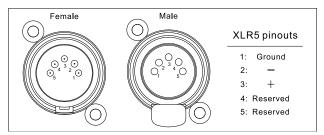
Connect the Console's DMX OUTPUT to the first fixture's DMX INPUT, then the first fixture's DMX OUTPUT to the second fixture's DMX INPUT and so on. It is recommended not to connect more than 32 units on a single DMX universe. On the last fixture's output connect a DMX terminator. (The terminator is a XLR connector with a  $\frac{1}{4}$  W and  $\frac{1}{200}$  resistor between the pin 2 and pin 3) as shown below:
